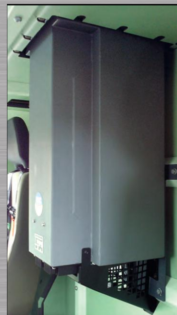
AFU 60m 3 /h integrated in SHERPA® vehicle
